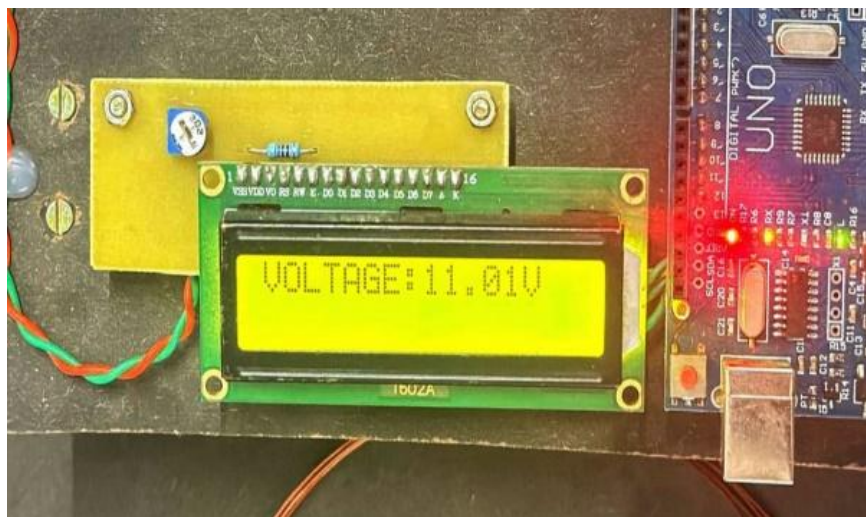
Figure 6. Output voltage due to mutual induction
